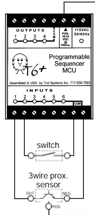
Electromechanical devices such as magnetic reed switches, limit switches, push button switches and pressure switches are wired with no regard to polarity (positive/negative).
