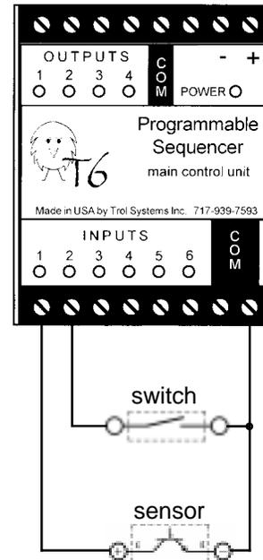
**Electromechanical** devices such as magnetic reed switches, limit switches, push button switches and pressure switches are wired with no regard to polarity (positive/negative).
