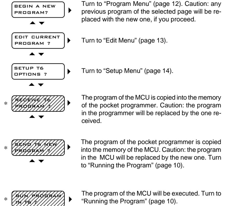
**\* Note:** The last three menu choices only appear if the pocket programmer is connected to the data port of the MCU *prior to applying power*. Be sure to remove the optional power pack (if used) from the programmer.
