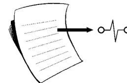
The selected output is turned on, turned off, or turned on for a selected amount of time. The function is now completed and the next line of the page is executed. Note: The page will begin the next line even if the output is timed on.
