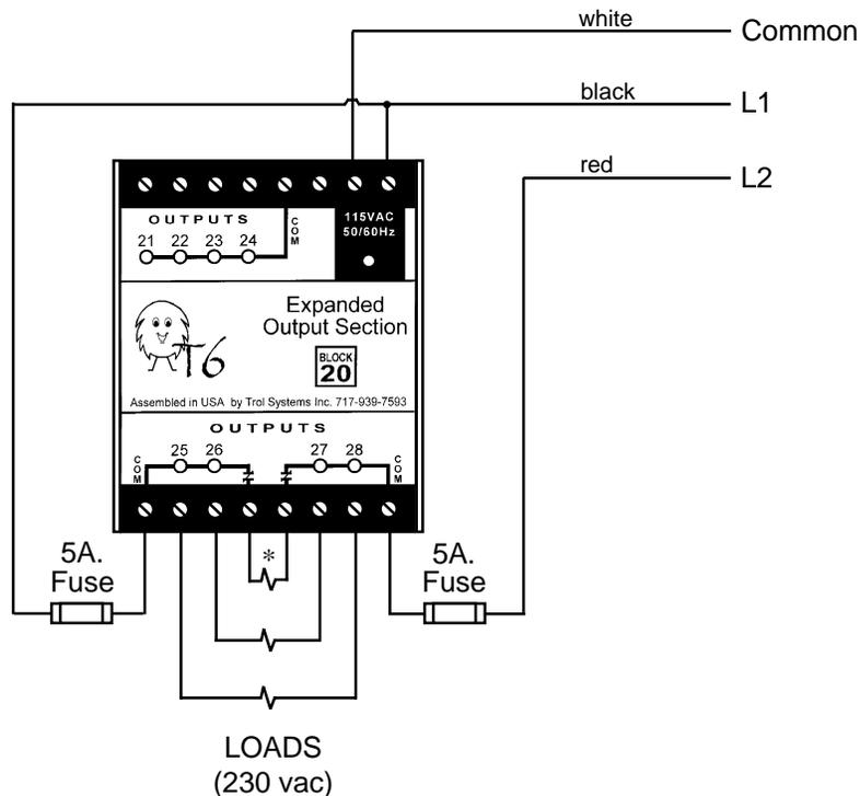
\* This load (connected to the normally closed contacts) is energized when outputs x6 and x7 are both turned off.
